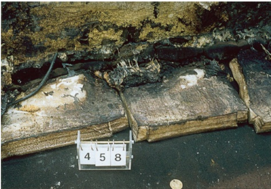
Exhibit 458, foam blocks recovered from wall of the drummer's alcove. Note corner cuts on each foam block, which assisted in matching them to polyethylene foam scavenged by Mickey Mikutowicz seven years before the fire. (Photo, William White)
